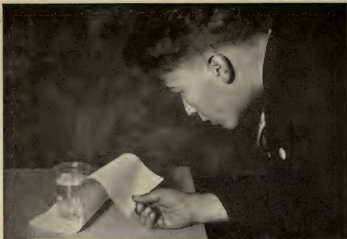
FIG. 34. When the paper is jerked out, the glass of water does not move.
